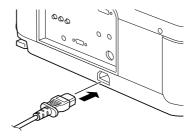
2. Connect the other end to a grounded electrical outlet.
