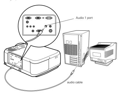
2. Connect the other end of the audio cable to the speaker or audio-out port on the Macintosh.
