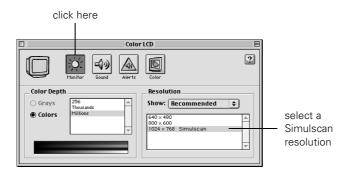
Select a Simulscan resolution as shown. (Allow a few seconds for the projector to sync up after making the selection.)
