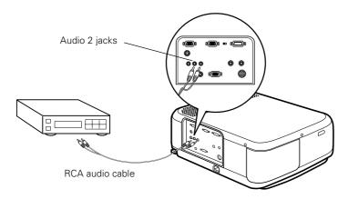
2. Connect the plugs at the other end of the cable to the audio output jacks on your video source.
