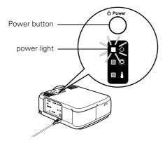
The power light flashes green as the projector warms up, and the projection lamp comes on in about 30 seconds. The power light stays green, and you may see a blue screen with the No Signal message displayed. This is normal.
