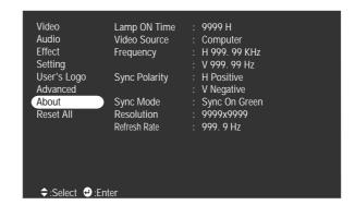
The life span of the lamp is about 1500 hours. If the number shown is close to 1500, make sure you have a spare lamp handy.
