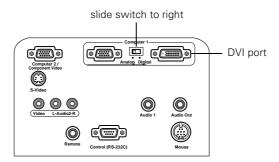
2. Using the tip of a pen or a small screwdriver, slide the Computer 1 interface switch to the right to select Digital. (If you need to use the projector's VGA port again, be sure to slide the switch back to the left.)
