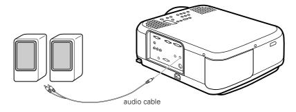
2. Connect the RCA plugs on the opposite end of the cable to the left and right jacks of your speaker or PA system.
