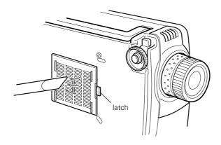
4. If the dirt is difficult to remove or if the filter is torn, replace it. Contact your dealer or call EPSON at (800) 873-7766 in the United States and Canada to obtain a new one.
