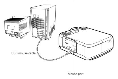
Disconnect your Macintosh's mouse cable. Connect the other end of the projector's mouse cable to the mouse or USB port on your Macintosh.
